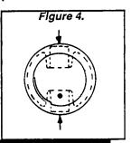
PISTON MINOR DIAMETER (GN190 & GN220) DESIGN DIAMETER: 2.747-2.748 inch (69.789-69.809mm)
